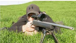
wide-angle lens offering approximately 20% more view than your standard one-inch models. It is a well-presented scope that has capped dial-up turrets with 1/4" MOA increments, plus a front mounted parallax ring that is easily adjusted for shooting at longer ranges. The Panamax has a Half Mil Dot reticle that was clear and easy to focus throughout the magnification range.
